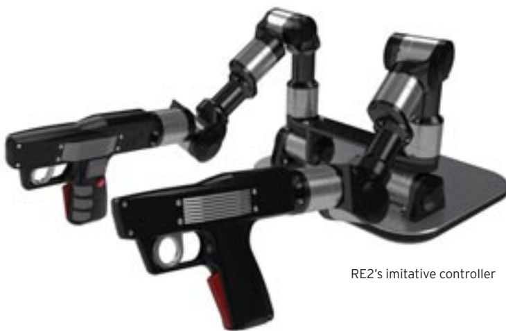
RE2's Highly Dexterous Manipulation System for ground-based EOD operations.
