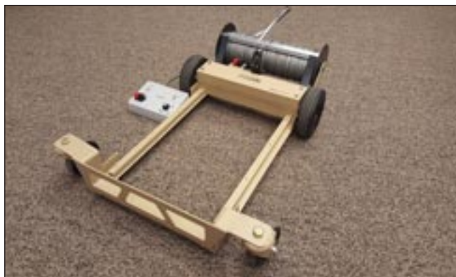
PAWN Vehicle-Borne Improvised Explosive Device (VBIED) robot
