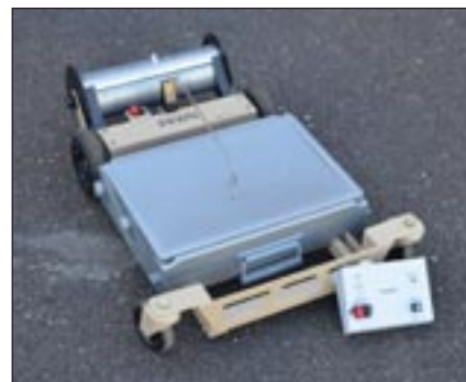
PAWN VBIED robot with Boot Banger water disruptor tool used to counter vehicle borne IEDs.
