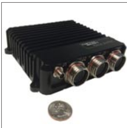
Parvus DuraCOR 310 Quad-core i.MX6 ARM miniature rugged mission computer.
