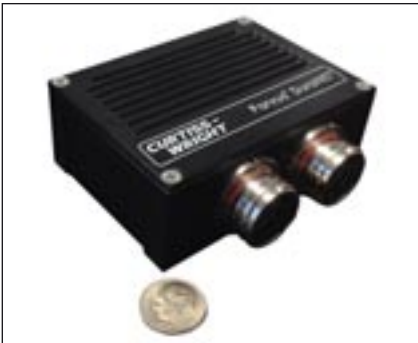
Ultra-small form-factor DuraNET 20-11 Ethernet switch supports network backbone upgrades on swap-constrained UAS platforms.
